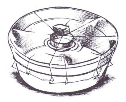
Place this apparatus in the sun. After some time, you will see drops of water forming on the under-surface of the plastic cover. The drops of water will drain into the small bowl. This is your distilled water. Do you see any similarity between what happens in your apparatus and the process by which we get rain?
