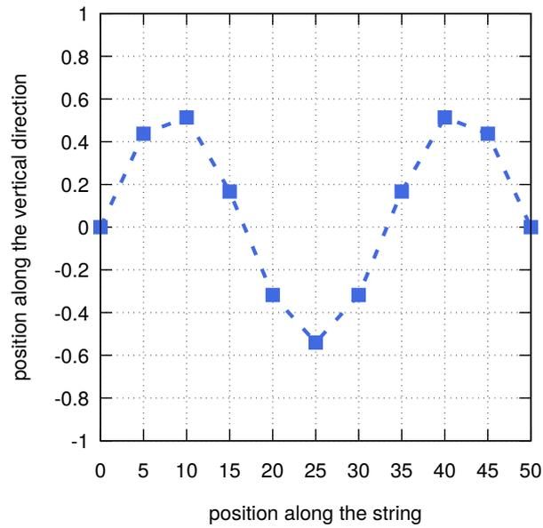
The motion of a vibrating string is the combined and synchronised oscillation of every point in the string. The difference between the motion of different points is in their speeds. Some points move fast, some slow. The ones that move slowly have small displacements, those that move fast have large displacements, but they all show periodic motion.
