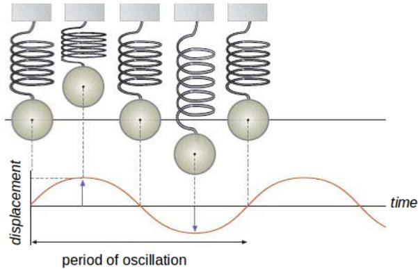
Understand various terms associated with an oscillation: frequency, amplitude.
